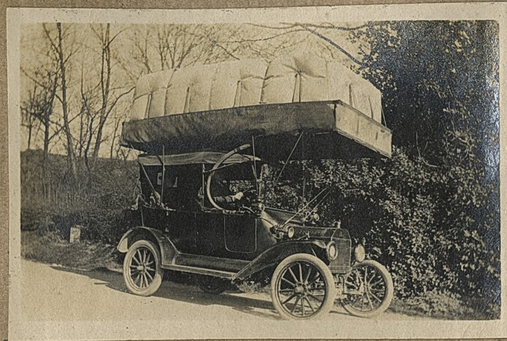
Motor-car driven by gas. The gas is stored in the bag above.
