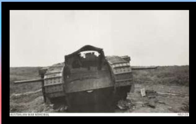
Figure 1. A British Mark I 'Male' tank knocked out during the final operations of the Somme battles of 1916 and photographed in April 1917. Similar 6-pounder tank guns were salvaged from derelict tanks by the 4th Australian Anti-tank Battery in May 1918 and mounted on improvised platforms as anti-tank guns. (AWM Collection H02120)
