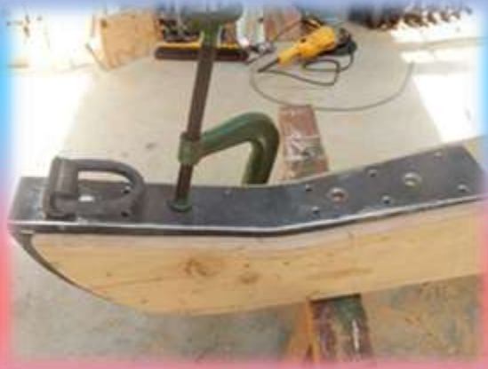
Trail plates being fitted, Nov. 2017.
