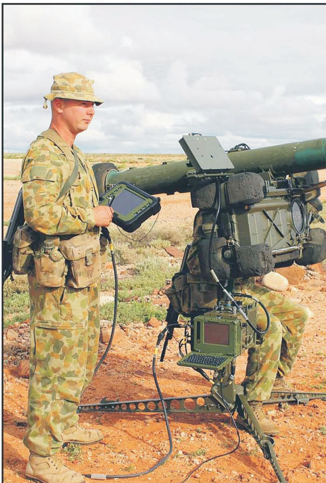
Ready to launch: LBdr Nathan Payne prepares to fire an RBS-70 missile.
