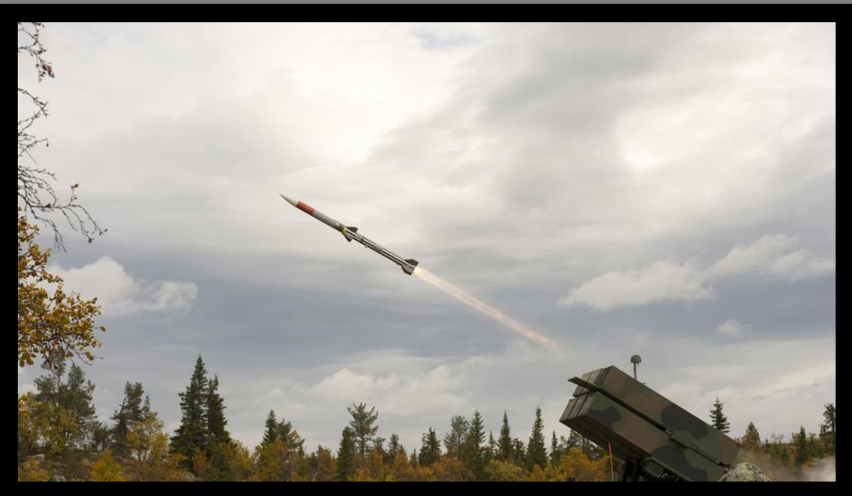
The NASAMS canister launcher firing an AMRAAM Missile
