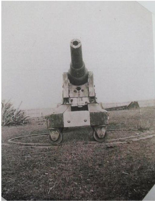
Above: An 80 pounder mounted on the traverse slide and timber sliding carriage, located on the racer rails with a timber fence to enclose the battery.
