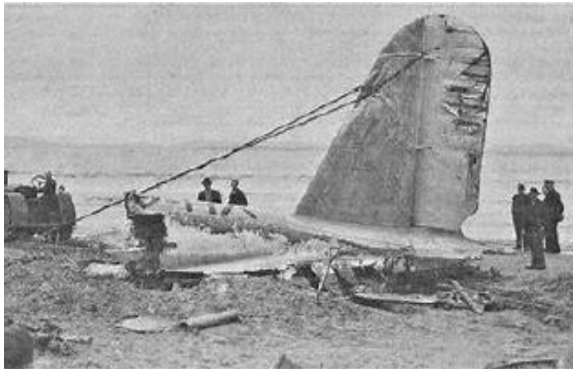
Wreckage of the aircraft's rudder and elevators. Source: Tasmanian Times
