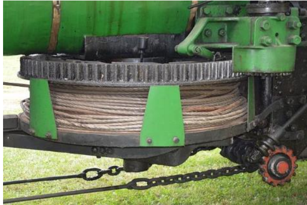
Image: Varga A. 3 Winch and steering detail of Fowler ploughing engine.
