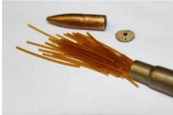
Figure 2. Forest H Barfield. Close-up of cordite filaments in a .303 British Rifle cartridge (manufactured in 1964). 7
